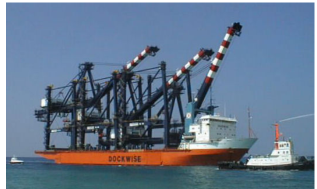
Figure 2: Dock Express 11 arriving at Freeport, Bahamas, with 3 container cranes with lowered superstructures
