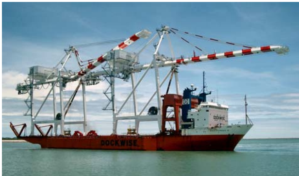
Figure 3: Dock Express 10 arriving at Laem Chabang, Thailand, with 2 new container cranes with booms down
