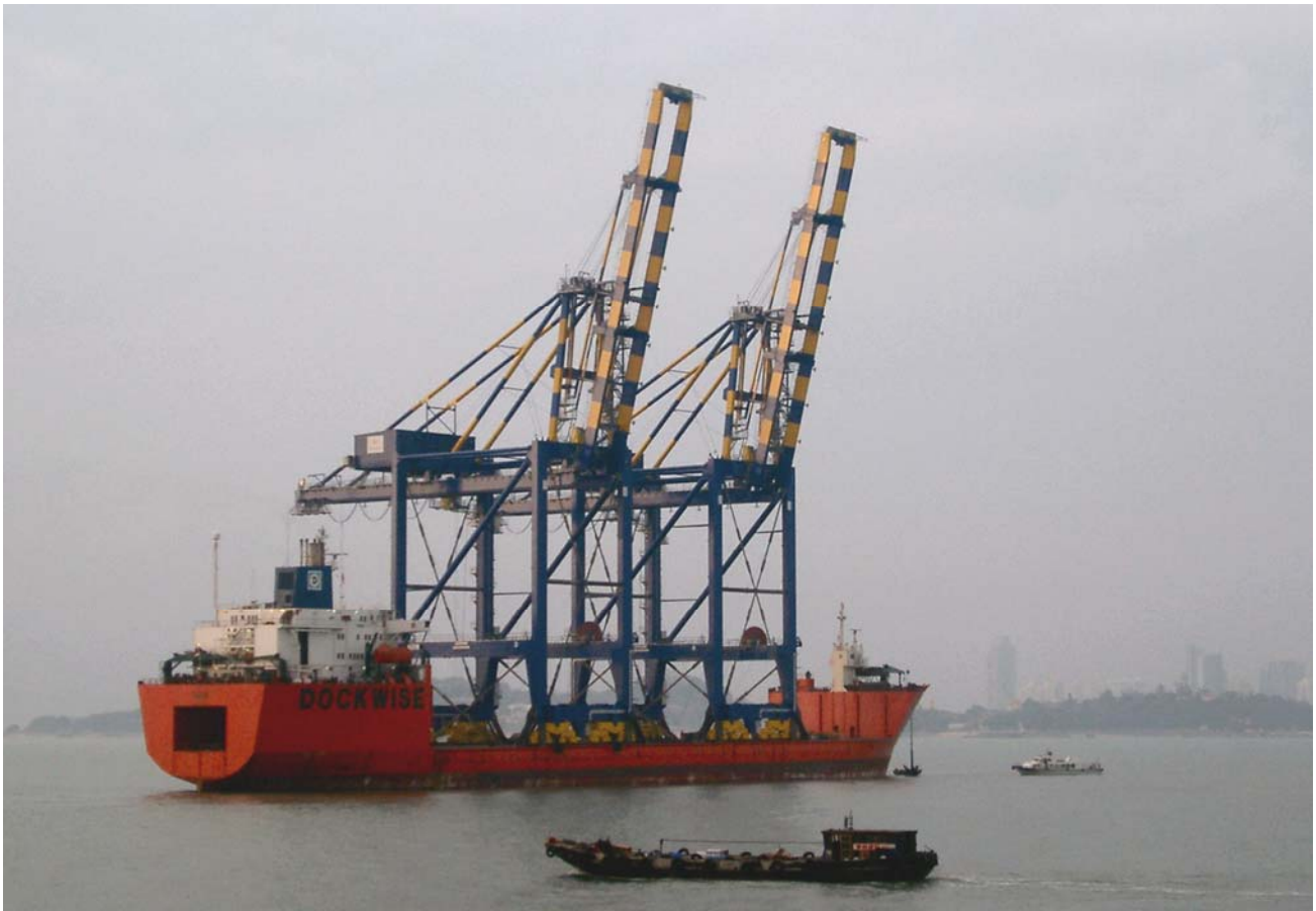
Figure 1: Heavy-lift ship Swan departing Xiamen, China, with 2 new container cranes for delivery to Mundra, India
