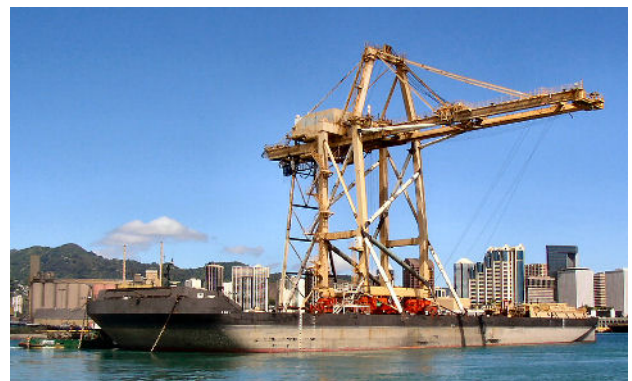
Figure 5: Barge Z Big 1 departing Honolulu with 1 old crane transversely stowed on deck
